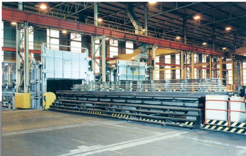
Aleris Aluminium, Koblenz / Germany plate length: max. 25,000 mm net charge: max. 60 t
