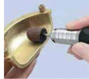
Seamless cap abrasives are easily pushed onto a rubber holder and can be quickly changed. Both the sides and ends can be used for polishing and finishing.
