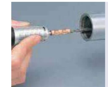
Wire lapping tools are made from banded piano wire. Ideal for burr removal and finishing of metals and plastics. They are also suited to polishing with abrasive compounds.
