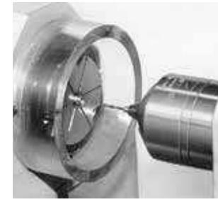
High rigidity and long clearance allow for high precision grinding of deep IDs.
