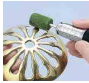
Felt bobs are made from 100% high quality wool. They are designed for superior finishing with abrasive compounds or with their embedded abrasives.
