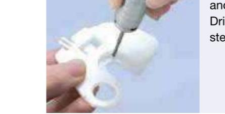
Tempered Steel Drills for plastics and woods. High Speed Steel Drills for steels and stainless steels, Carbide Drills for PCB, FRP.
