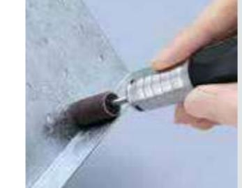
Seamless abrasive cartridges are easily pushed onto a rubber holder and can be quickly changed. They are ideal for finishing wide open areas.
