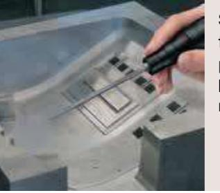
Special electroplated diamond files of Nakanishi's ultrasonic polisher "SHEENUS ZERO". Ideal for fine burr removal and rough finishing.
