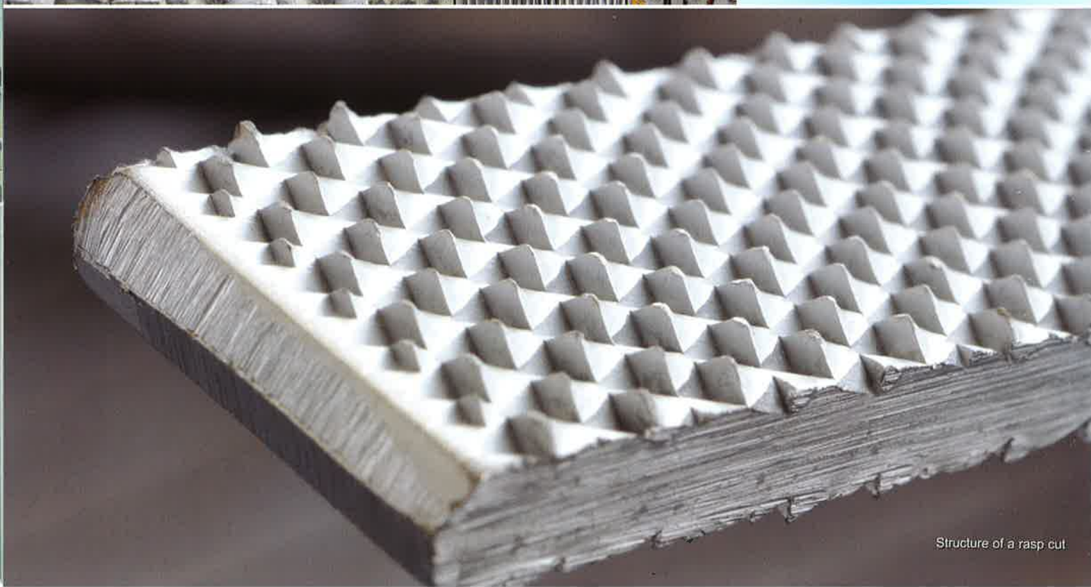
Macro photograph showing rasp cut details
